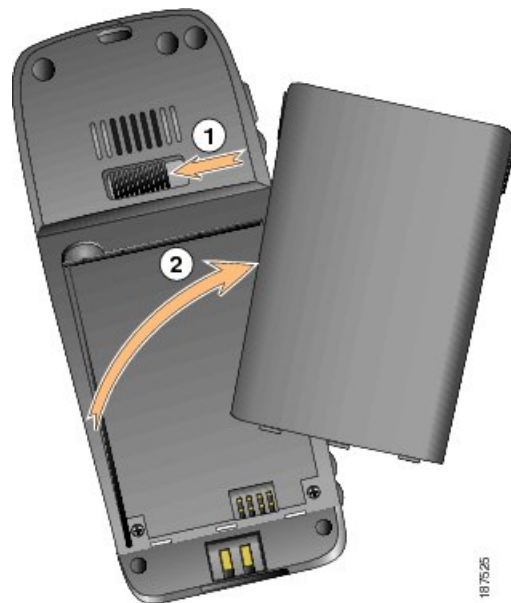
Figure 4: Remove cover to install the battery
