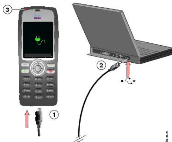
Figure 8: Charge the phone battery using the USB cable and PC
