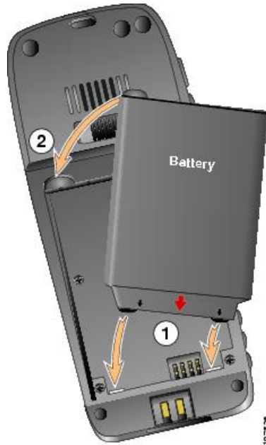
Figure 5: Install the battery
