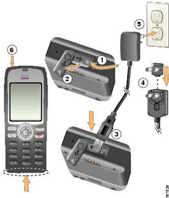
Figure 7: Charge the phone battery
